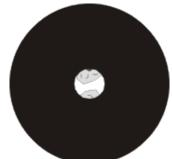
Open the field diaphragm until it just disappears out of the field of view.
