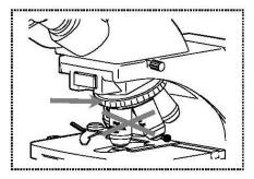
When rotating the nosepiece you must always make sure that the objective which is about to be positioned in the beam path does not touch the object holder. This can lead to significant damage to the objective lens.
